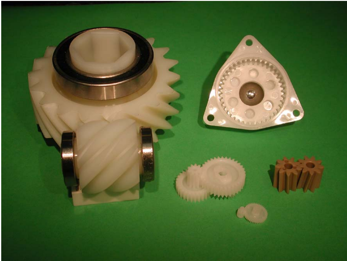
Molded gears can be made in many forms and varied sizes.
