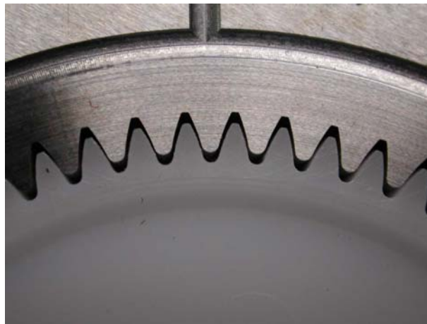
The Involute Shrinkage of a Molded Gear
